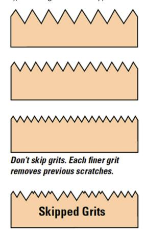
Once the mistake has been made to proceed to the next grit too quickly, it becomes impossible to correct this mistake without going back to the original coarse grit. Proceed slowly through each; making sure that the entire valley is removed.
