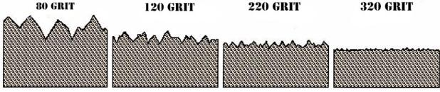
\*Note TWO things shown in the Diagram. The size and depth of the 80 grit scratches, AND how the 120 grit scratches (the highs and the lows) are all BELOW the previous grit; as are the 220 & 320 grit diagrams. Transitions should always look like this regardless of grit.
